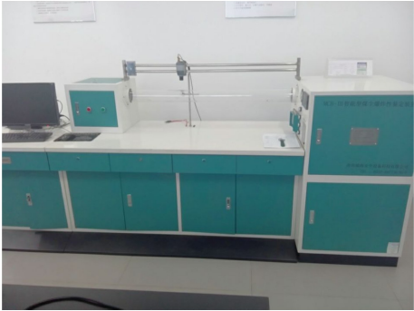
图 1 煤尘爆炸性鉴定装置 Fig. 1 Identification equipment of coal dust explosibility
