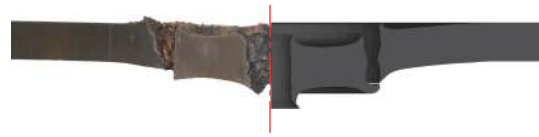
图 17 偏心环锥罩的试验结果和数值模拟结果对比 Fig. 17 Comparison between experimental and numerical simulation results of eccentric liner
